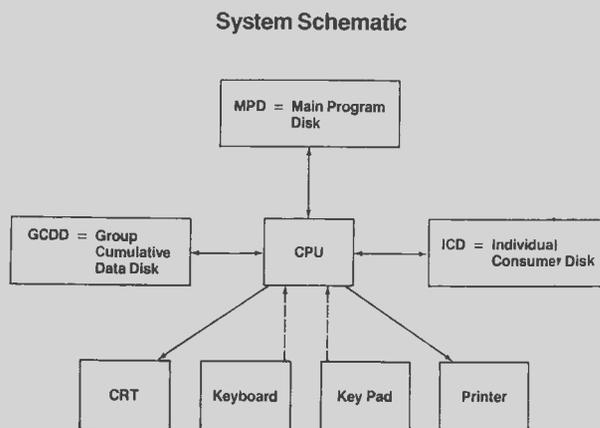
Fig. 1. A schematic diagram of the interrelationships between the Central Processing Unit (CPU), the disk drives for each major function and the input/output devices. The CRT (Cathode Ray Tube) or VDU (Video Display Unit) is actively used during data input, review and editing while the printer is used primarily for final reporting.
