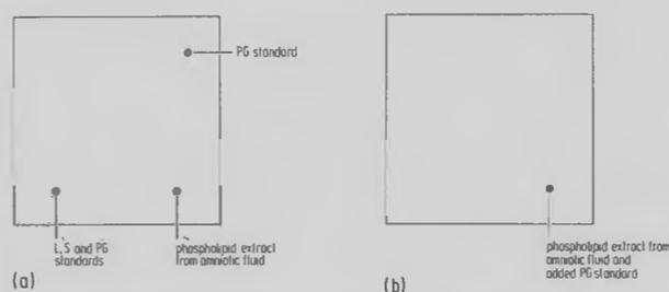
Fig. 1. Preparation of thin layer chromatography plates for analysis of amniotic fluid phospholipids. (a) Sample sheet. (b) Reference sheet with phosphatidylglycerol (PG) added to amniotic fluid extract.
